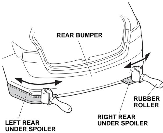
16. Using a rubber roller, apply firm pressure, especially at the ends, to set the adhesive.
