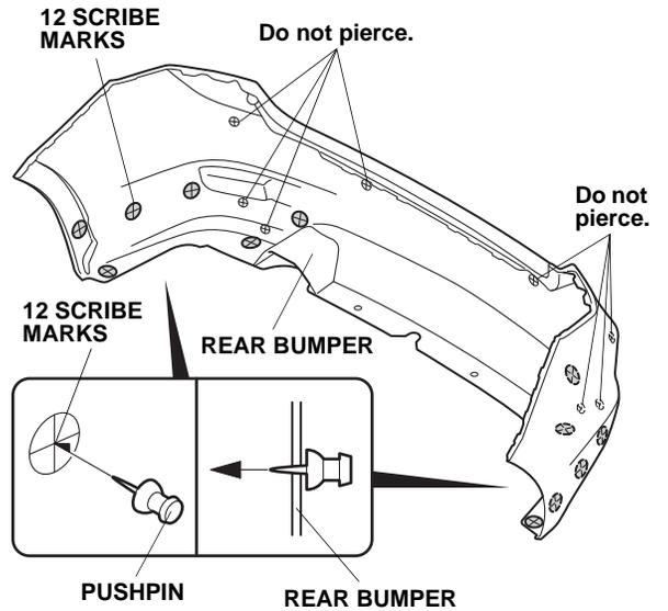
3. While wearing eye protection, drill the 12 pierced marks with a 3 mm drill bit. Enlarge the holes with a 10 mm drill bit.
